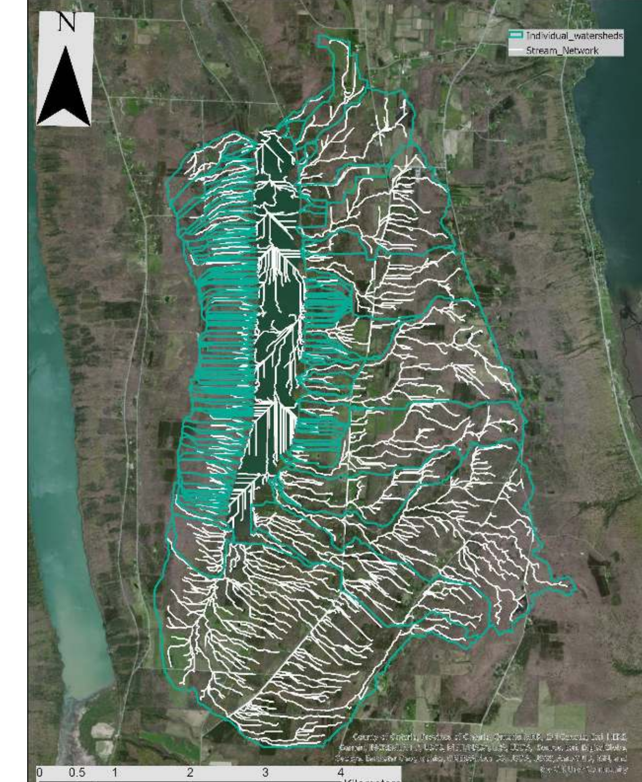
Figure 4. Stream networks and individual watersheds from flow accumulation grid and pour points
