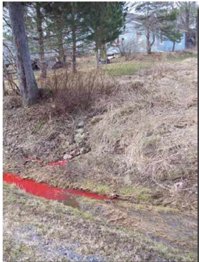
Dye testing is one of many tools used to determine onsite wastewater system failures.
